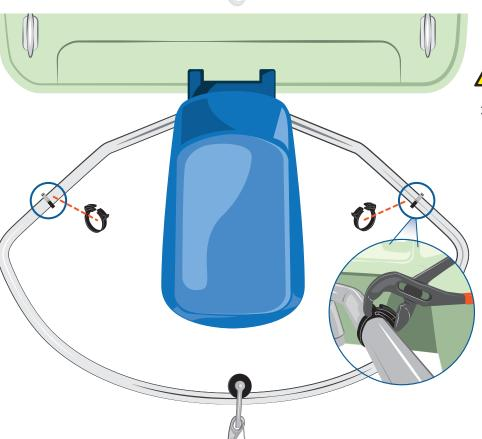
Tighten existing stopper on one side and add one additional stopper next to it.
