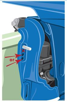
1c. Determine where to drill your TurboSwing holes using the base plate as a guide. Leave 1-2 holes in between the original and new bolts.
