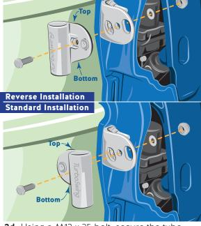
**2d.** Using a M12 x 35 bolt, secure the tube holder to the base plate and tighten using locking nut.
